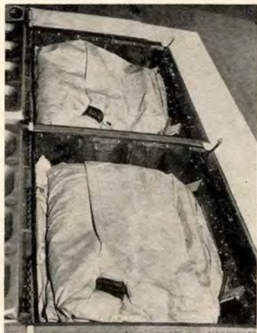
Rafts installed in wing trailing edge compartment. Unvented gas pressures can build up enough to cause door to pop open, loss of raft.
