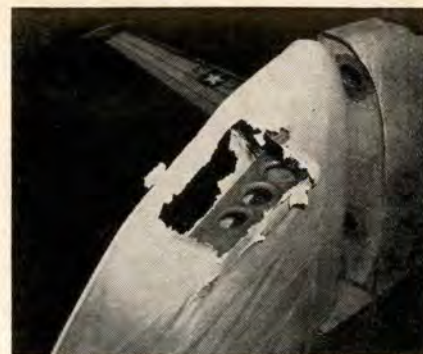
Note damaged rudder of C-124. Aircraft was struck while flying below 10,000 feet.
