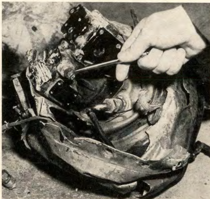
Get-home-itis and impatience, finally a do-it-yourself mod job to get engine started ended pilot's career. Investigator points to jerry-rigging repair job.
